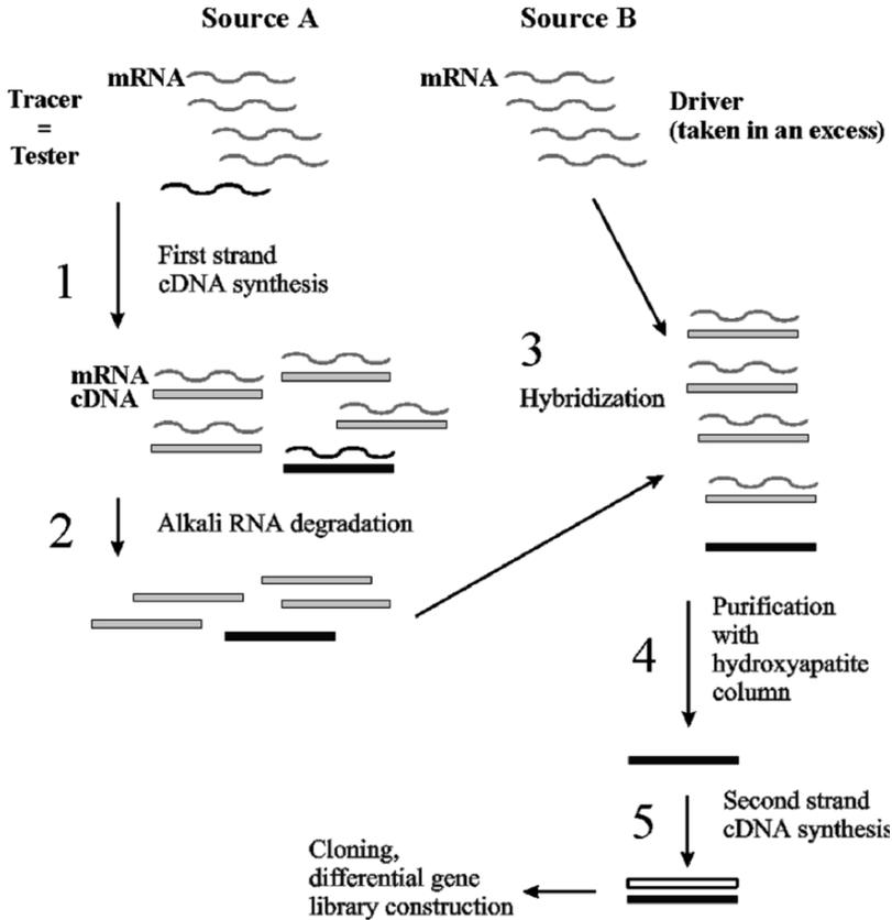
Figure 2. cDNA/mRNA subtraction scheme, utilizing alkali RNA degradation at stage 2.
